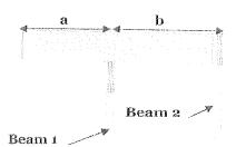
Use "a" or "b", whichever is greater, to determine the joist size. Use "a" + "b" to determine the size of Beam 1 and the post footing size for the posts supporting Beam 1. Use joist length "b" to determine both the size of Beam 2 and the post footing size for the posts supporting Beam 2.
